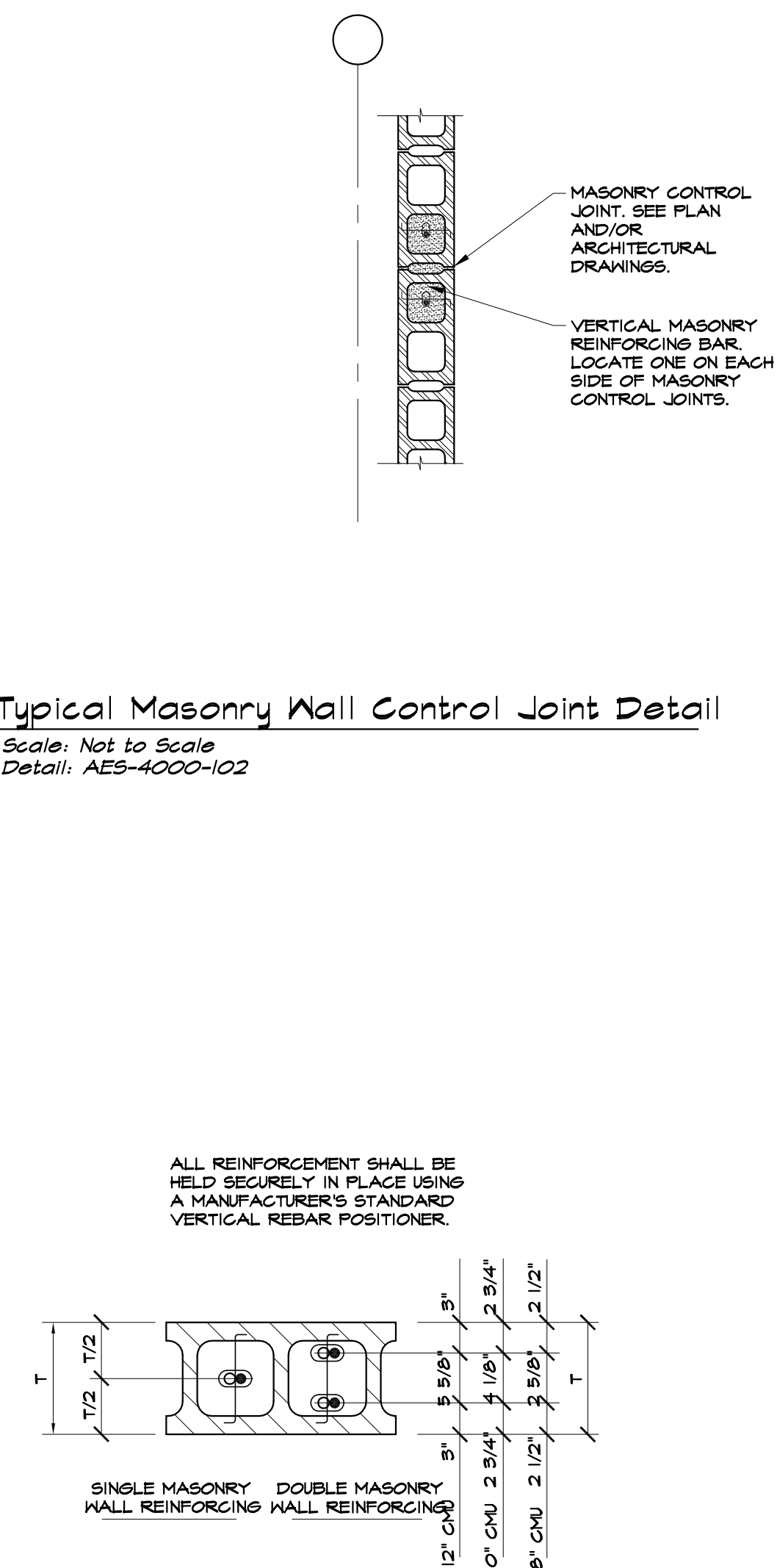
2 Typical Masonry Wall Reinforcement Detail
